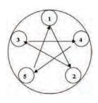
5 bolt wheel tightening pattern.
