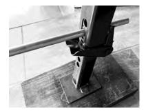
Stabilizer jack adjustment bar, passing through both sets of holes on stabilizer jack.
