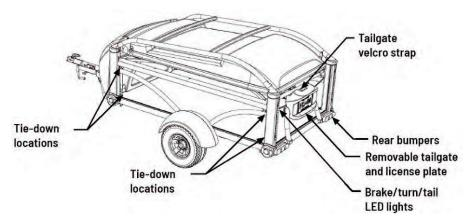
\*Note: Additional tie-down options can be achieved by securing to the lip, on the underside of the frame.
