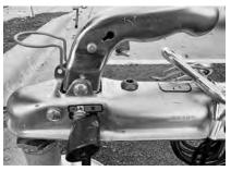
Coupler with indicator showing positive connection to ball.
